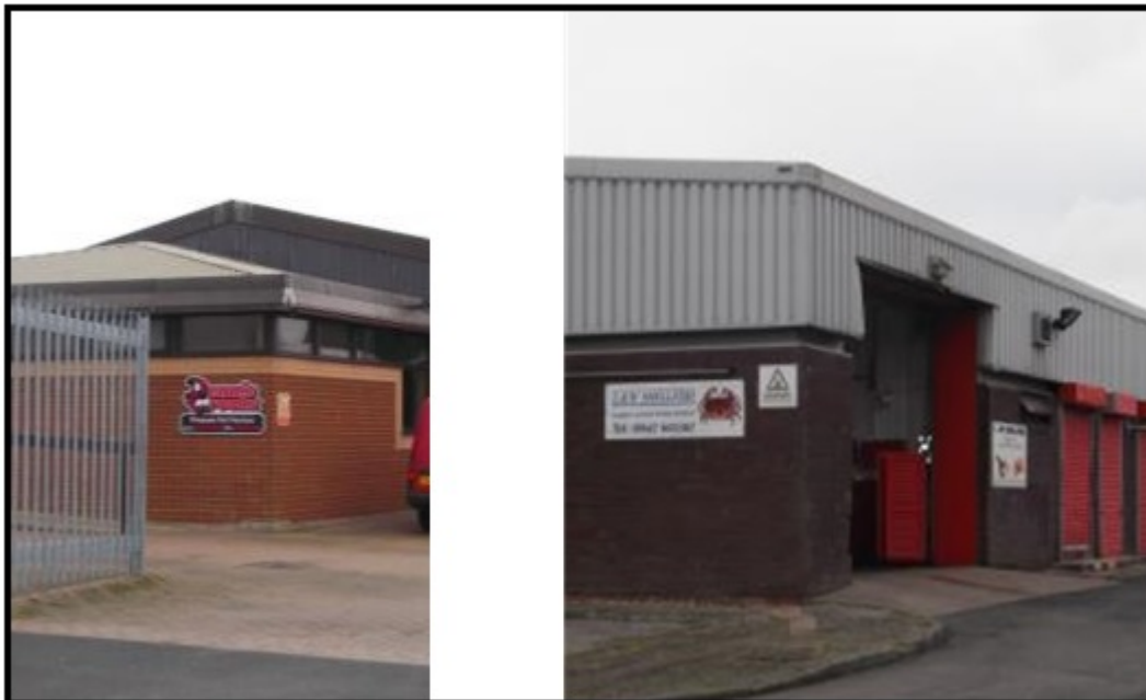
Figure 9.1 One non-illuminated sign on the front face of the building is most appropriate to avoid clutter. Where additional warning signs are required they should if possible be away from the business name to avoid clutter
